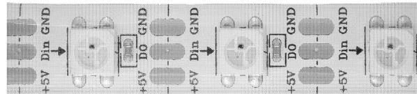
The components of an LED strip are surface-mount soldered to a flexible printed circuit board (PCB). If you bend the strip at too sharp of an angle it can break the solder joints and since each LED is fed from it's neighbor, a break like this will make ever LED after it stop working as well. This kind of break can also happen if you twist a strip, so be sure to keep them flat.
